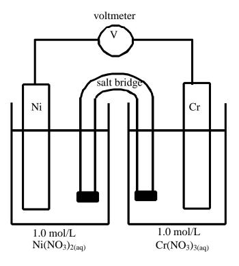
$Cr_{(s)} \rightarrow Cr^{3+}_{(aq)} + 3 e^{-} E^{\circ} = +0.74 v$  $Ni_{(s)} \rightarrow Ni^{2+}_{(aq)} + 2 e^{-} E^{\circ} = +0.25 v$
