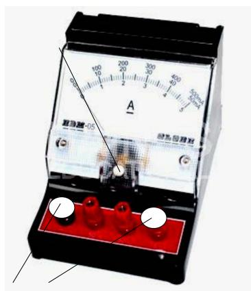
The same current is being read at three different settings. Show how the accuracy improves as we move towards the right scale for this small current.
