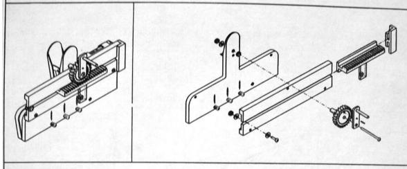
Crank: When you turn its arm, the <u>crank</u> drives the pinion, making it rotate (transmits rotational motion).
