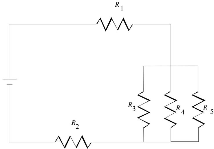
$$R_1 = 25 \Omega \quad R_2 = 15 \Omega \quad R_3 = 20 \Omega$$
