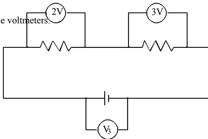
4. In the following electric circuit, one of the two resistances is  $4.0 \Omega$ . The other resistance, " $R$ ", is unknown. The voltage of the power source is  $12 \text{ V}$  and the electric current from the source is  $4.5 \text{ A}$ .
