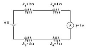
6. The following electric circuit consists of two resistors  $R_1$  and  $R_2$  and a power source. Using an ammeter, you measured the current
