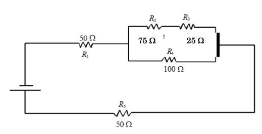
If the voltage of the power source is 150 V, what is the potential difference across  $R_3$ ?
