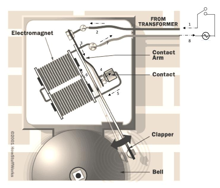
The above model of a doorbell uses an electromagnet and a contact arm. The electron flow is revealed by the 8 numbered broken-lined arrows in the diagram.
