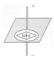
**a.** Apply the left hand rule. Have your thumb point up because the electricity is flowing straight (like your thumb) from (-) to (+). Notice that the rest of your fingers point left. This is the direction of the magnetic field in front of the wire. The field is caused by the moving electrons.
