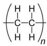
In this case(polyethylene) the monomer is C<sub>2</sub>H<sub>4</sub>
