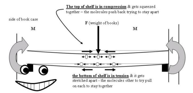
a beam is said to "smile" in bending: the top is in compression & bottom is in tension
