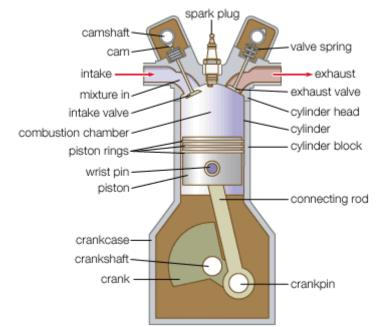
d) Is the link between the crank and piston direct? No. there is a connecting rod between them.
