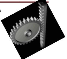
If you fix the pinion(circular gear) to an axle and attach a base to the rack, by turning the pinion the rack will move up and lift the base and whatever weight is placed on it.
