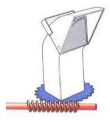
1. Use the velocity (speed) ratio and mechanical advantage to explain why it makes sense to use a worm gear system for a snow blower.
