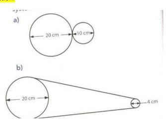
Make the back gear 5 cm, so that the ratio becomes 20/5 = 4/1.
