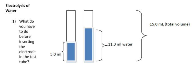
The test tubes have to be filled with water and acid to speed up the process.
