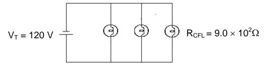
Each CFL in this circuit costs \$17.00 and has a lifespan of 6 000 hours.
