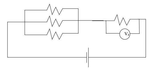
Since this is an overall series circuit, the current passing through  $R_4$  is equal to the current just before it splits at the parallel part. But the parallel part only has 1/3 of the resistance compared to  $R_4$ . Why? If three identical resistors are in parallel their resistance will be divided by 3.
