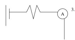
Connect a third a wire to the ammeter's red button that reads **5 A**. (This is an important step. Attaching it elsewhere could damage the instrument.)
