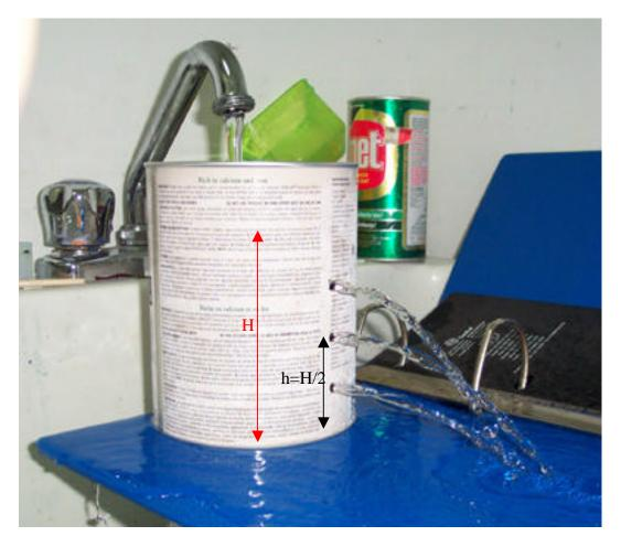
One would expect that the water near the lowest exit point is under the most pressure, so that it should travel the furthest. But it does not. The picture reveals that the water from the middle-hole is traveling about a centimeter past the farthest reaches of the other two projectiles, which are practically identical.
