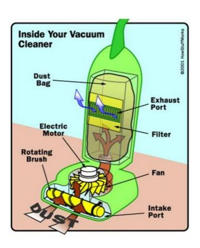
cleaner. This allows atm. pressure to push air and dust from the outside into the bag. The air molecules go through the bag's microscopic pores, but most of the dirt gets trapped inside the bag. .
