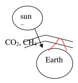
The arrow represents visible light going right through the greenhouse gases, which are invisible, so they do not prevent the earth from receiving energy. But once the earth warms up, some of the infrared(see red curve) that tries to escape back into space is absorbed by CO<sub>2</sub> and CH<sub>4</sub>.
