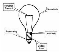
Which of the above substances used to make this light bulb are *insulators*?
