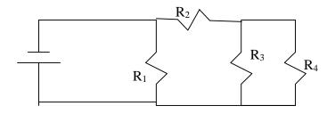
If the total voltage is 12V, find the voltage across each resistor.
