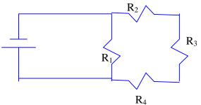
$R_2,\,R_3$  and  $R_4$  are in series. Being identical resistors, they have the same voltage, so since  $V_2+V_3+V_4=Vt$
